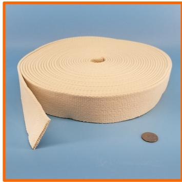
This is a widely used and universal tape for making gaskets, especially where a rough or uneven surface or flange exists. The tape is a fiberglass base with a special white rubber formulation coating. The tape is tacky, and has a plastic film surface covering that is removed before installation. The tape will stick to itself once the film is removed.
