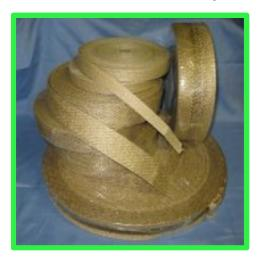
Vermiculite coated fiberglass tape is manufactured from texturized fiberglass yarns then coated with Vermiculite, a 100% inorganic dispersion. Certified to meet the requirements of ASTM E 162, ASTM E 662 & SMP 800-C for surface flammability, smoke and toxic gas generation.
