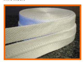
This is a widely used and universal tape for making gaskets, especially where a rough or uneven surface or flange exists. The tape is a fiberglass base with a special white rubber formulation. The tape is tacky, and has a plastic film surface covering that is removed before installation. The tape will stick to itself once the film is removed.
