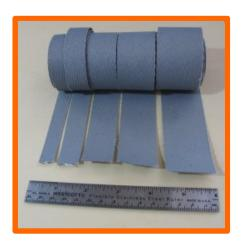
This tape is made from silicone rubber coated fabric; and is typically used as a gasket material or to wrap hydraulic hoses, lines, cables and wiring when a sleeve cannot be installed. The tape has an internal woven fiberglass fabric base which allows only a very minimal amount of bias elongation and negligible elongation along its width and length. (1-side coated tapes such as part number T-FG-SR provide higher elongation).
