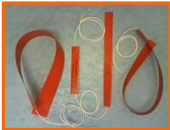
These heaters are commonly used to prevent condensation from forming in outdoor equipment such as motors and enclosures. Can be embedded under sleeving on piping to regulate process temperatures.
