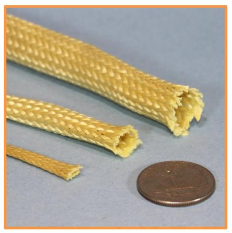
Kevlar sleeve is soft and pliable, highly flexible.
