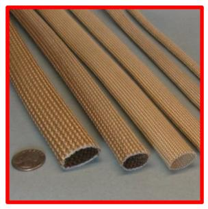
This Braided fiberglass sleeve is fabricated from high quality type E fiberglass that will not burn and will withstand continuous exposure to temperatures of 1200°F / 648°C. The sleeve is heat treated before being saturated.
