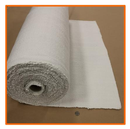
This is a widely used and universal fabric for making gaskets, especially where a rough or uneven surface or flange exists. The fabric is a fiberglass base with a special white rubber formulation. The fabric is tacky, and has a plastic film surface covering that is removed before installation. The fabric will stick to itself once the film is removed.
