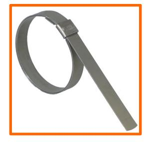
Preformed Stainless Steel Twice-Around clamps are the strongest clamps available for firesleeve or hose assembly. Use our Firesleeve Clamp Tool for closing and locking these clamps. Clamp widths available are 0.25", 0.375", 0.55", 0.625" and 0.75" wide. 0.25" wide clamps are type 201 stainless steel. 3/8" / 0.375" through 3/4" / 0.750 clamps are available in type 201 or 316 Stainless Steel and Galvanized Carbon Steel.
