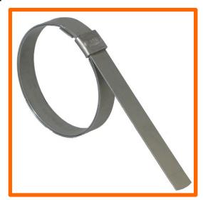
Preformed Stainless Steel Twice-Around clamps are the strongest clamps available for firesleeve or hose assembly. Use our Firesleeve Clamp Tool for closing and locking these clamps. Clamp widths available are 0.25", 0.375", 0.5", 0.625" and 0.75" wide. 0.25" wide clamps are type 201 stainless steel.
