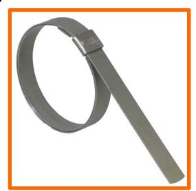
Preformed Stainless Steel Twice-Around clamps are the strongest clamps available for firesleeve or hose assembly. Use our Firesleeve Clamp Tool for closing and locking these clamps. Clamp widths available are 0.25", 0.375", 0.5", 0.625" and 0.75" wide. 0.25" wide clamps are type 201 stainless steel. 3/8" / 0.375" through 3/4" / 0.750 clamps are available in type 201 or 316 Stainless Steel and Galvanized Carbon Steel.
