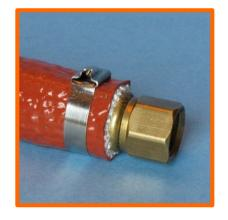
Free-end or twice-around clamps are used to secure firesleeve over hoses at the fitting. Twice-around clamps offer better tensile strength than free end clanps and provide superior clamping of hydraulic hoses onto fittings.
