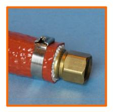
Free-end or twice-around clamps are used to secure firesleeve over hoses at the fitting. Twice-around clamps offer better tensile strength than free end clamps and provide superior clamping of hydraulic hoses onto fittings.
