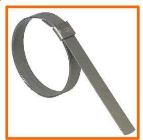
Preformed Stainless Steel Twice-Around clamps are the strongest clamps available for firesleeve or hose assembly. Use our Firesleeve Clamp Tool for closing and locking these clamps. Clamp widths available are 0.25", 0.375", 0.5", 0.625" and 0.75" wide. 0.25" wide clamps are type 201 stainless steel.
