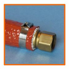
Free-end or twice-around clamps are used to secure firesleeve over hoses at the fitting. Twicearound clamps offer better tensile strength than free end clanps and provide superior clamping of hydraulic hoses onto fittings.
