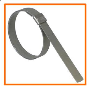
Preformed Stainless Steel Twice-Around clamps are the strongest clamps available for firesleeve or hose assembly. Use our Firesleeve Clamp Tool for closing and locking these clamps. Clamp widths available are 0.25", 0.375", 0.5", 0.625" and 0.75" wide. 0.25" wide clamps are type 201 stainless steel. 3/8" / 0.375" through 3/4" / 0.750 clamps are available in type 201 or 316 Stainless Steel and Galvanized Carbon Steel.
