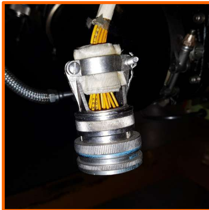
Tape used as a backshell clamp bushing
